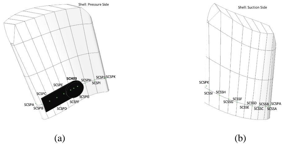
Figure 4-5. Stator blade monitor points on shell streamline pressure side (a) and shell suction side (b).
