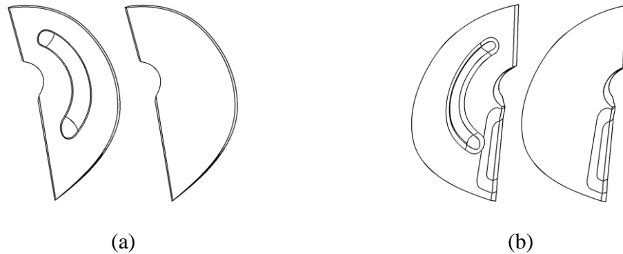
Figure 3-7. Blade designs with and without ribs for impellers (a) and turbines (b).
